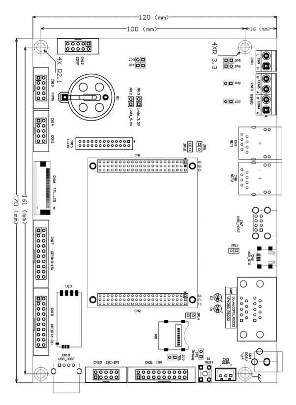
ESMARC Evaluation Board Mechanical Drawing – Top Side (unit: mm)
