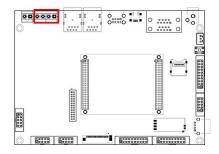
Pins of RS485 interfaces are contained in CN1
