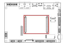
An ESMARC Compute Module can be firmly connected with the EVB through CN1 and CN2. For the pin-out of the ESMARC module, please refer to the applicable ESMARC module datasheet. The pin B1 in CN1 is blanked out so that ESMARC module can be plugged in correct orientation. It is recommended to use M2 size screws to fasten ESMARC module with the carrier board if required.
