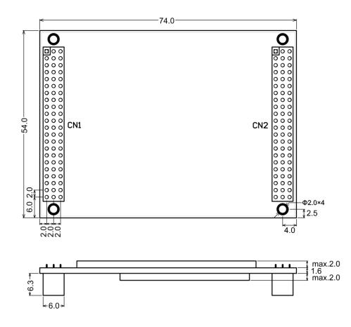
ESMARC Computer Module Size (unit: mm)
