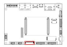
Connector type: 1x 40 FPC socket, 0.5mm pitch
