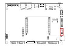
Connector type: 2x5 IDC, male header pin, 2.54mm pitch
